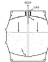
**Figure 6: The dispense of beer from a pressurized keg.**
