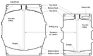
**Figure 4: Typical metal kegs for pressurized beers.**
