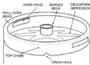
**Figure 7: The top dome of a typical cylindrical metal keg.**
