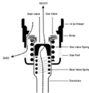
**Figure 5: A typical extractor.**
