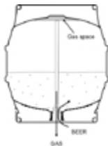
**Figure 8:** Filling a keg through the gas-ports of the extractor.
